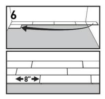
4. To start the second row, use 1/4 or 1/3 of a full-width plank (You can use the left-over piece from the last plank of the first row). Ensure that the end joints of the planks from the second row and the first row are staggered by at least 8 inches. With the cut side against the wall, insert the tongue into the first plank of the first row and drop it until is lying flat over the underlayment.
