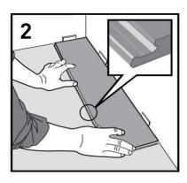
2. Begin placing the planks for the first row at the left-hand corner of the room. Place the first plank with the two cut sides facing the wall. The groove should face outwards in both directions (see image above). Remember to use 1/4" spacers around the perimeter.
