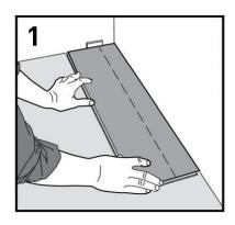
1. Start the first row. Cut each of the planks length-wise with the previously calculated measure. (Don't worry if the plastic insert falls off the groove. You can easily place it back). Trim off the tongue on the short side of the first plank.
