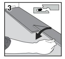
3. Put the second plank by pushing the tongue against the groove of the first plank. Use pressure on the short edge until you hear a snap or click. Continue doing the same with the rest of the planks of the first row. Cut the last plank to finish the row.
