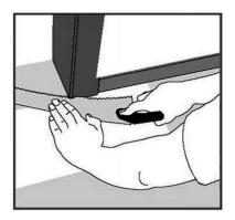
**Doors:** When fitting planks around door trim its necessary to slide the plank under the trim. To secure the right cut, turn a plank upside down and place it on the floor up to the door frame. Then place a handsaw flat against the plank and simply cut through the frame. Remove the cut out and vacuum away debris.
