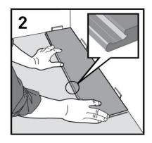
2. Begin placing the planks for the first row at the left-hand corner of the room. Place the first plank with the two cut sides facing the wall. The groove should face outwards in both directions (see image above). Remember to use 1/4" spacers around the perimeter.
