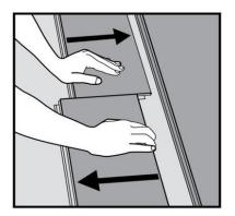
Our Waterproof Floors can be easily disassembled to replace planks during installation and in case of damage. Separate the whole row by carefully lifting up and slightly knocking just above the joint. Disassemble the planks by sliding horizontally only.
