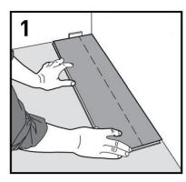
1. Once the underlayment is laid down, start with the first row. Cut each of the planks length-wise (with the previously calculated measure). Don't worry if the plastic insert falls off the groove, you can easily place it back in. Trim off the tongue on the short side of the first plank.
