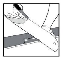
Install around radiator pipes by drilling holes in a plank around 3/4" larger than the diameter of the pipes. Cut out the plank (with the thinnest blade possible) as per the image above. Install the plank as per normal. Glue the cut-out piece back again.
