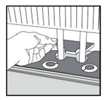
Glue the cut-out piece to the plank itself only. Do not glue it to the underlayment or sub-floor. You must always allow the floor planks to move in all directions after the installation is complete.
