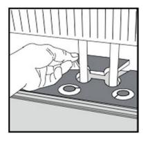
Glue the cut-out piece to the plank itself only. Do not glue it to the underlayment or sub-floor. You must always allow the floor planks to move in all directions after the installation is complete.
